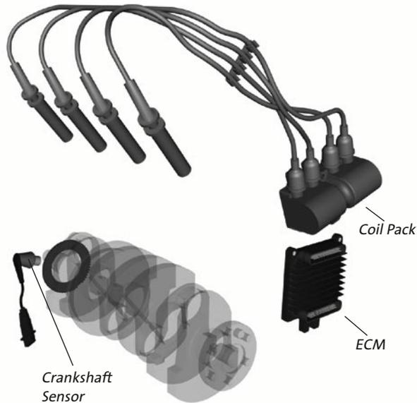
The crank-triggered, waste spark ignition system uses a crankshaft position sensor, coil pack, and available ECM to replace the distributor and coil used in conventional ignition systems, so servicing of distributor caps and rotors is eliminated. Crankshaft position is precisely determined directly from the crankshaft, resulting in improved spark accuracy. The OEM-established spark timing cannot be changed by the end user.
